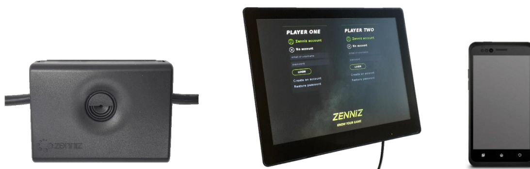
Figure 1. Components of the Zenniz system (from left to right): microphone; touchscreen display; auxiliary device (smartphone). Not to scale.
