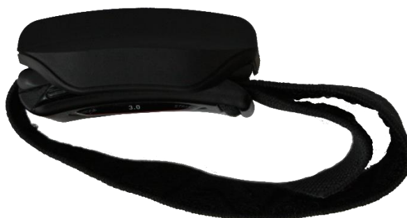
Figure 4. Battery pack fitted to the WHOOP 3.0 for charging in-situ .
