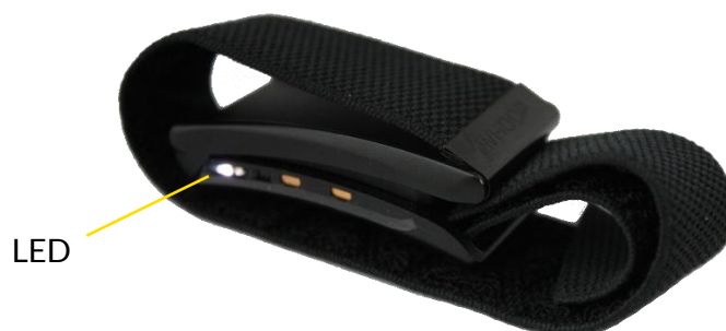
Figure 3. White LED indicating pairing mode is active.
