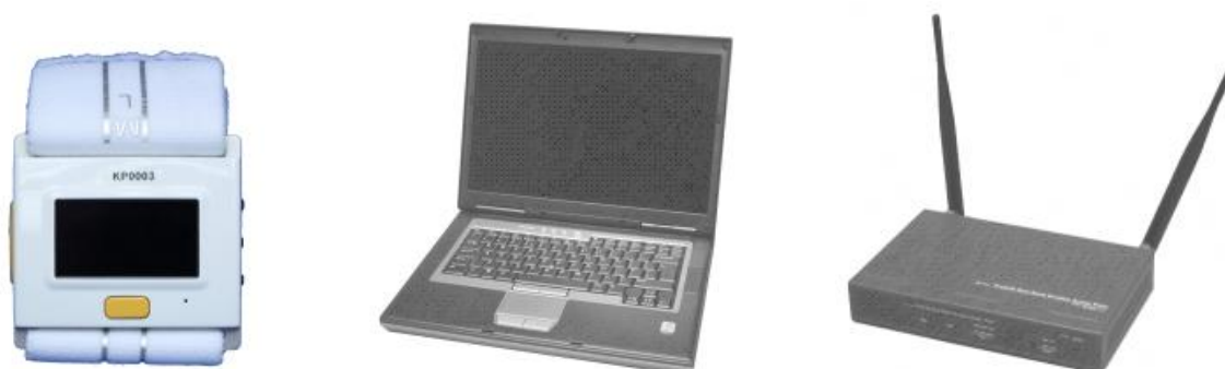
Figure 1. Components of the KITRIS system (from left to right): KIT device; auxiliary device (laptop); internet access to KITRIS Server (router).
