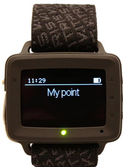
Figure 3. LED confirmation of point input (green light signifies point won by the user).
