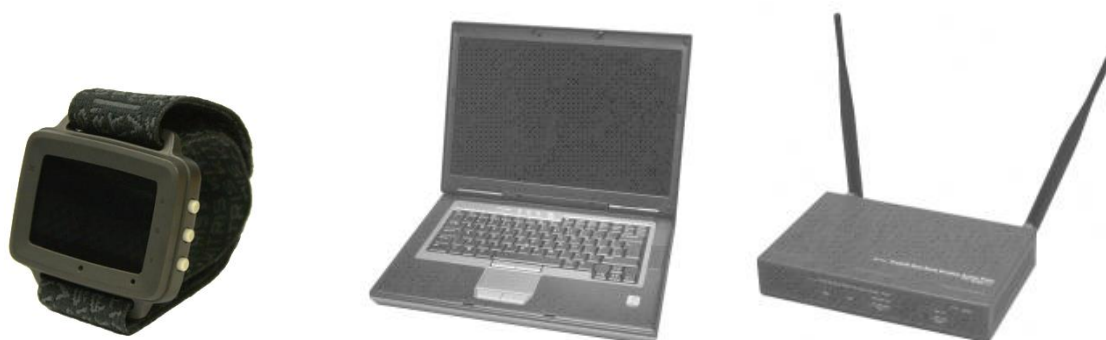
Figure 1. Components of the KITRIS KIT BIA system (from left to right): KIT device; auxiliary device (laptop); internet access to KITRIS server (router).
