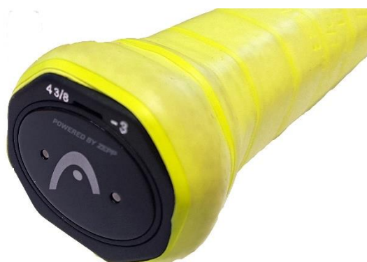
Figure 2. HEAD Tennis Sensor attached to the butt of a racket.
