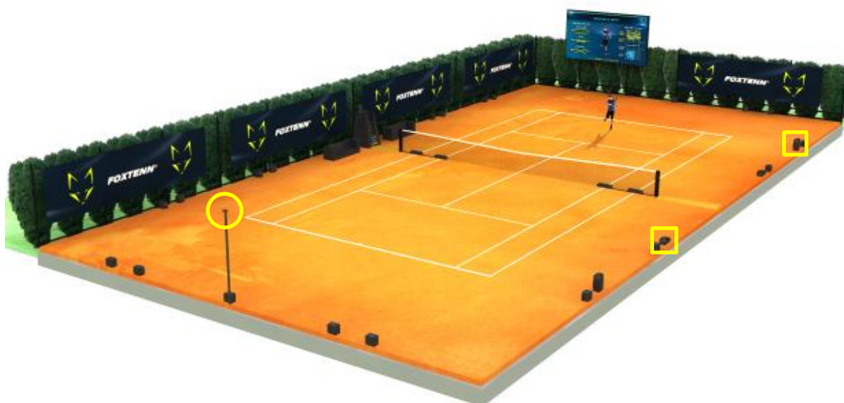
Figure 2. Cameras (circled) and laser scanners (marked by squares) fixed around the court.
