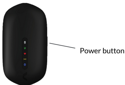
Figure 2. Catapult Vector S7 pod power button and status LEDs.
