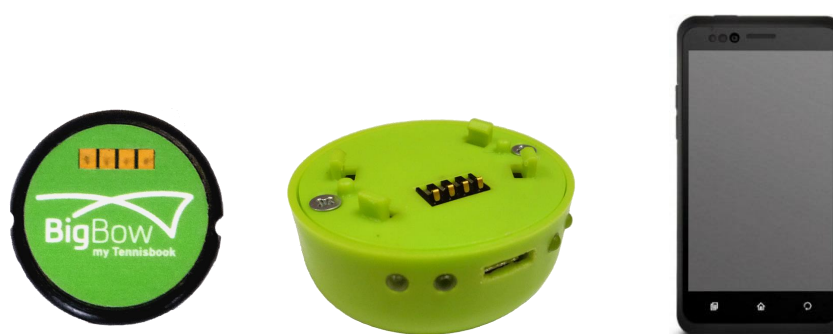
Figure 1. Components of the BigBow Champion Sensor system (from left to right): Champion pod; charger; auxiliary device (smartphone).
