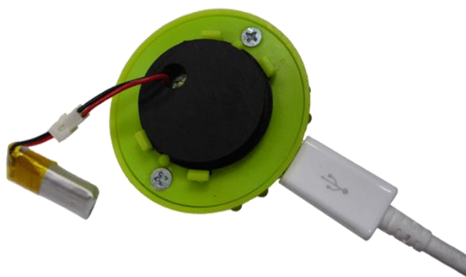
Figure 4. Champion pod connected to charger and charger connected to an auxiliary device (e.g. laptop) via USB cable.
