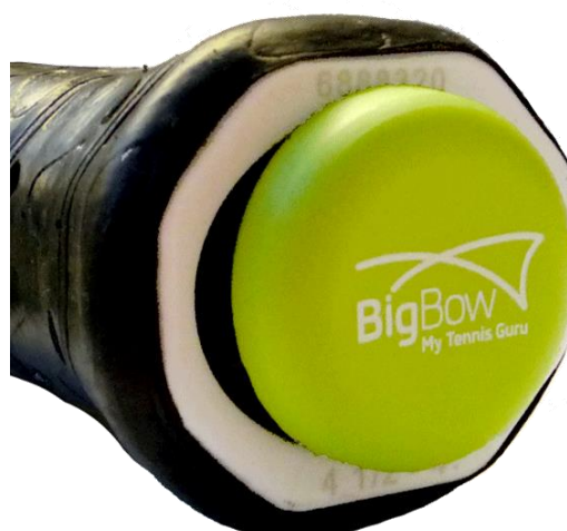
Figure 2. Champion pod, fitted with protective cover, attached to the butt of a racket.
