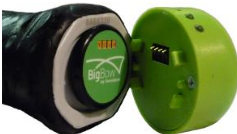
Figure 3. Disconnecting charger from Champion pod.
