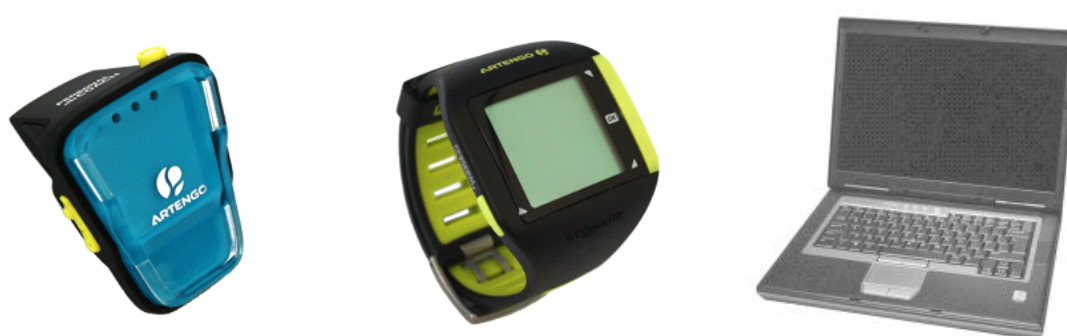
Figure 1. Components of the Artengo Personal Coach system (from left to right): pod; watch; auxiliary device (laptop).
