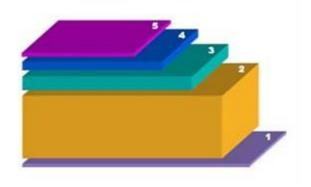
Consisting of rubber bound in polyurethane, polymeric surfaces can be cast in situ, or provided in prefabricated rolls. These surfaces need a flat concrete or asphalt substrate.
