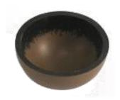
A vulcanising rubber solution is applied to the edge of the buffed half shell.
