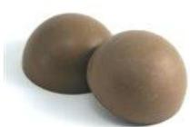
The half-shells are removed from the press, joined together in a sheet by the 'flash', which has spread out of the moulds during the forming.
