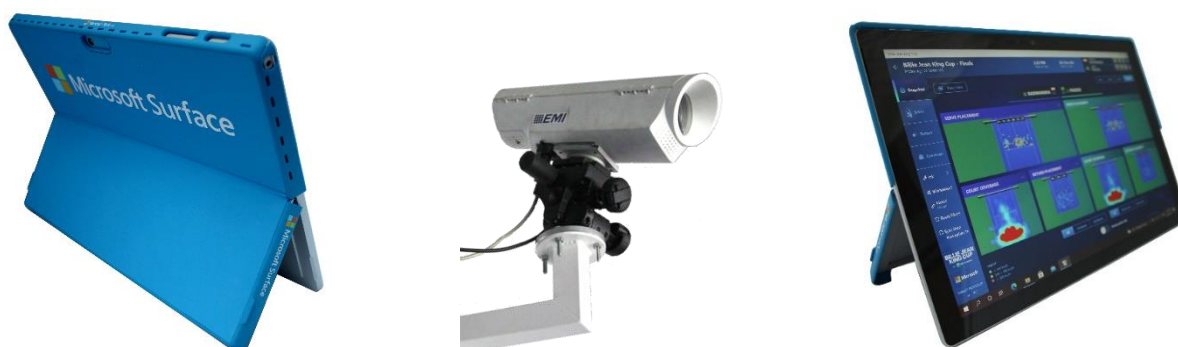
Figure 1. Components of the Billie Jean King Cup Match Insights App system (from left to right): Tablet (for live scoring), video camera, Surface device (with Billie Jean King Cup Match Insights App). Images are not to scale.
