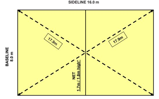
**Note:** All court measurements shall be made to the outside of the lines.
