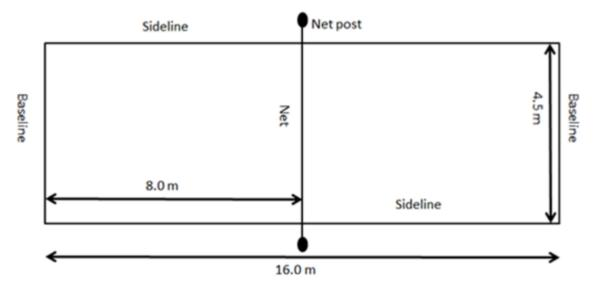
Note: All court measurements shall be made to the outside of the lines
