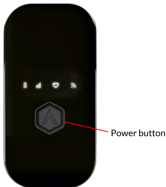
Figure 2. STATSports APEX pod v3.2 power button and status OLEDs.
