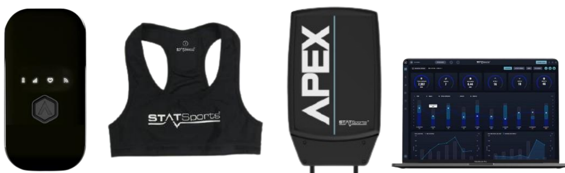
Figure 1. Components of the Apex system (from left to right): STATSports Apex Pod v3.2; STATSports Vest, STATSports Apex Beacon, auxiliary device (laptop). Not to scale.
