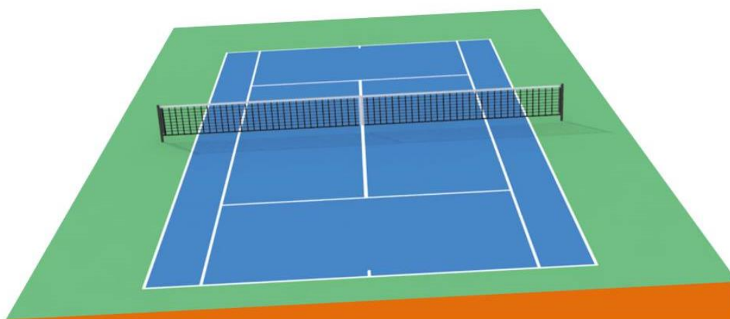
Figure 6. Preferred orientation of slope (side-to-side), if necessary.
